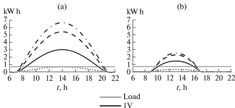
**Fig. 1.** Daily curves of load and electric energy generation from SPPs of different arrangements as of June 22 (a) and December 21 (b).
