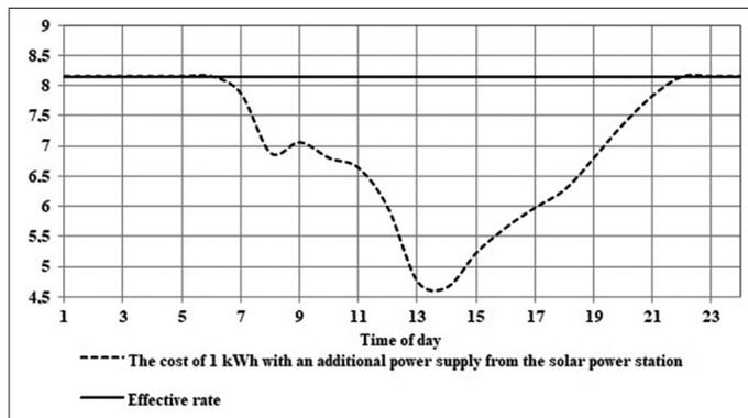
peak and is due to the nature of the arrival of the solar radiation flux to the collecting surfaces of the southern orientation equally located in space. During the functioning of the solar power plant, the cost of electricity is reduced by 7.9%–14.1% in the morning hours, and by 32.5%–44.7% at high solar activity.
