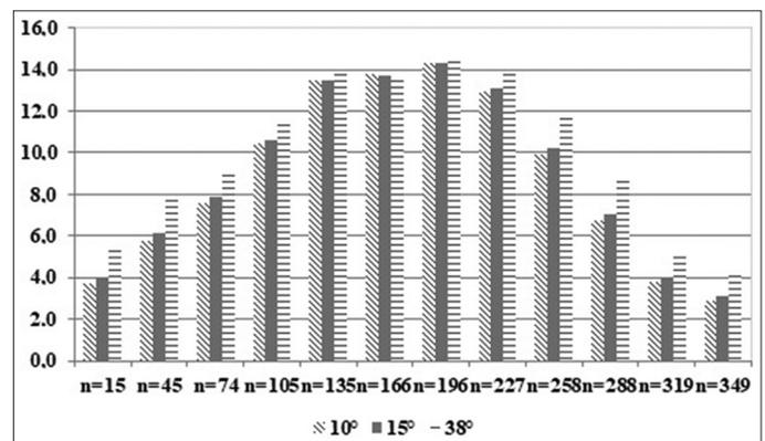
**Figure 4:** Dependence of the cost price of the electric energy generated by a solar power station depending on the number of photovoltaic panels
